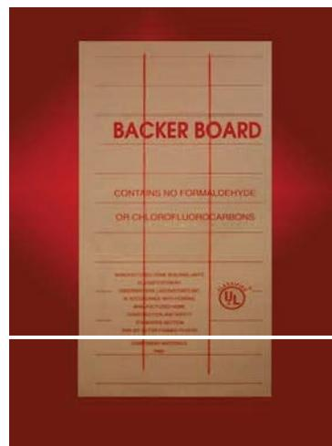
Vertical stud location lines are placed on the product at 16" and 32" from the leading edge of the board. Product installed in the wall area of the home shall always be installed with vertical stud location lines being up and down on the house.
